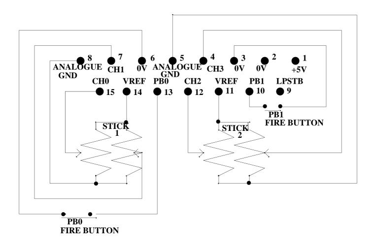
The potentiometers shown in the diagram should be of approximately 10k in value and the fire buttons are simple switches which are open when at rest. The actual construction of the joystick itself is entirely at the users discretion but it is recommended that they are self centering.
